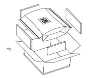
4. Place vacuumed bag into an outer box and place EPE on 4 sides of the bag for protection.
