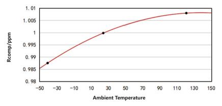
Figure 7-1. RCOMP Temperature Characteristic Curve
