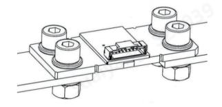
Figure 8-2. 8436 Shunt Connection Diagram
