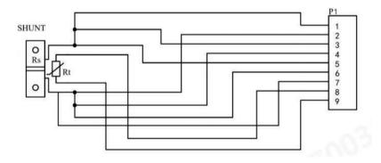
Figure 8-1. PCB Structural Diagram
