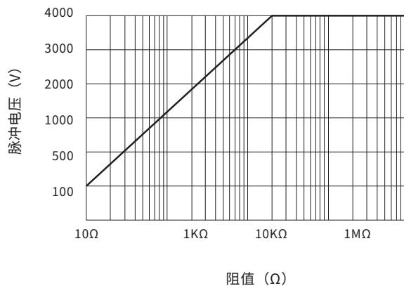
脉冲负载额定值符合IEC 60115-1,4.27; 12 $\mu$ s/50 $\mu$ s;
